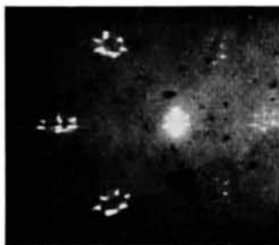
Fig. 1. Laue photograph of a \text{CdI}_2 crystal. Incident radiation makes an angle of 25^\circ 40' with the c axis; a axis vertical, Cu white radiation; camera radius 3 cm. Diffraction spots in reflexion alone are shown.
